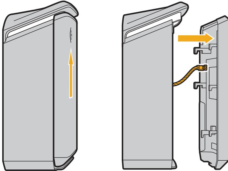
5. Press the locking tab of the cable connector to release the cable from the network board on the interior of the faceplate, and carefully pull the cable away from the network board.
