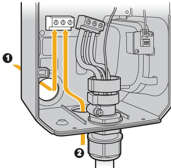
2. Strip the ends of the conductors 0.4 in (11 mm).
