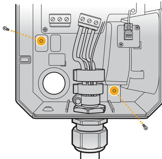
4. Torque each screw to 12 in-lb (1.36 Nm).
